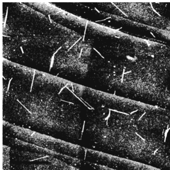
Figure 8. Large-scale tapping mode image ( 2 \times 2 \mu\text{m} ; scale bar 500 nm) of a layer of dendrimer 1 prepared from a dichloromethane solution (20 \mu\text{g/mL} ) after annealing the sample at 96 ^{\circ}\text{C} for 30 min.
