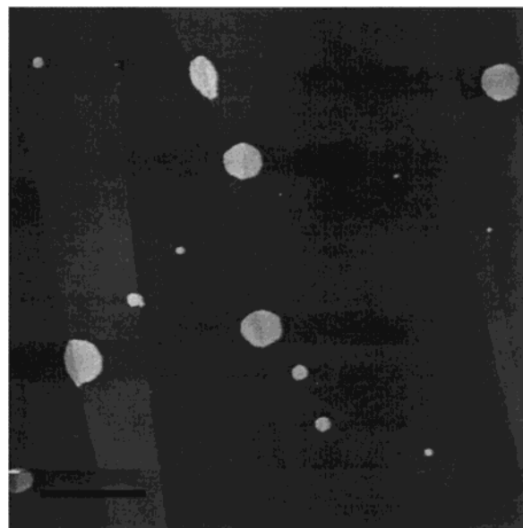
Figure 9. AFM tapping-mode image of a sample prepared from a 20 \mu\text{g/mL} solution of dendrimer 1 dissolved in dichlorobenzene on graphite ( 5 \times 5 \mu\text{m} ; scale bar 1 \mu\text{m} ).
