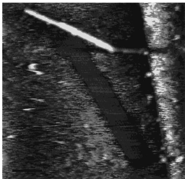
Figure 13. Dendrimer 2 layer prepared from 2 \mu\text{g/mL} dichloromethane solution ( 615 \times 615 nm, scale bar 100 nm). A region consisting of parallel rows with a spacing of 6 nm can be seen.
